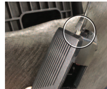
Connect the Power Supply Connector to the Power Supply
