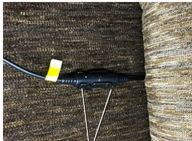
Hand Wand Connection with Locking Cover
