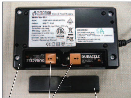
Power Transformer (2) 9-Volt Alkaline Batteries Battery Cover
